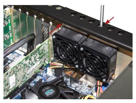
**4.** Insert the plug of the fan power supply cable into the appropriate plugs on the motherboard, see picture below.
