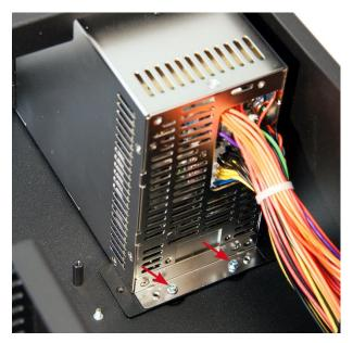
**4.** Loosen 2 screws each on the left and the right side, which are used to fix the bar (1) and remove the bar.
