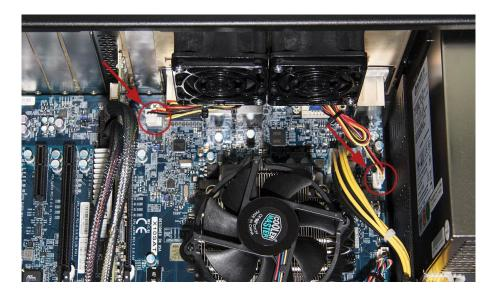
5. The guide pins on the plug ensure a proper position of the connection.
