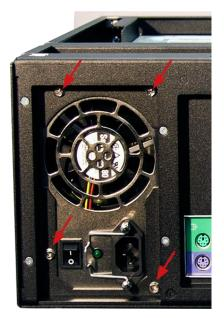
Loosen 2 screws each on the left and the right side, which are used to fix the bar (1) and remove the bar.
