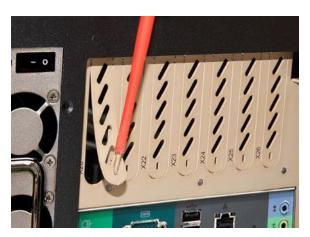
**3.** Above the slot, there is a screw in an opening, which is used to fix the card later. Loosen the screw and remove it.
