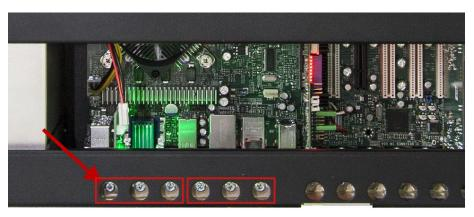
**3.** Insert the fan module on the inner side on the rear cover, for this purpose push the bent slot bracket onto the rear cover. Fasten the fan with the screws removed before.
