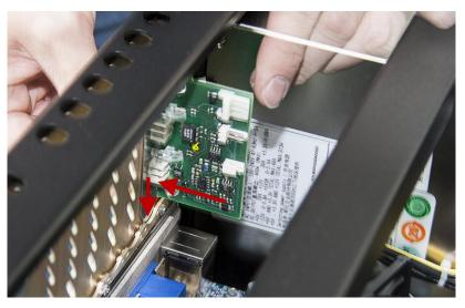
5. Fasten the card with the screw removed in step 5.
